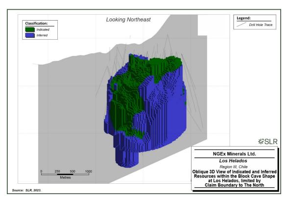
Figure 6: Los Helados Indicated and Inferred Blocks Within the Block Cave Shape
